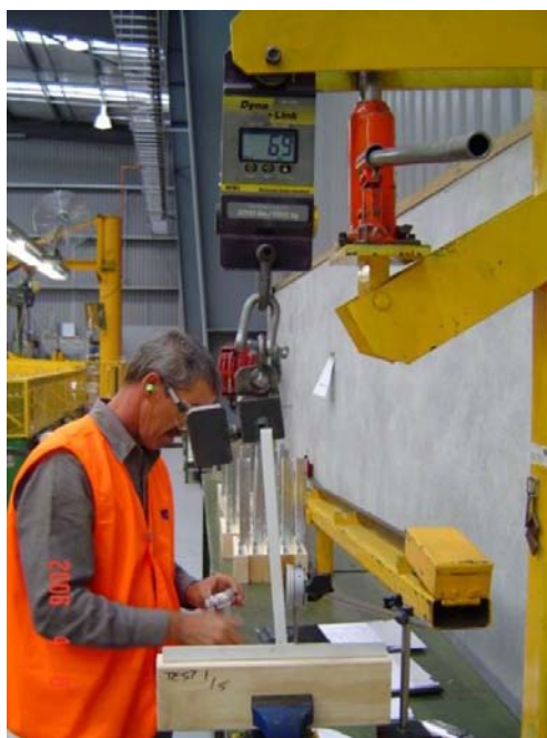
Figure 2: Photograph of Teg Tab tensile test set-up.
